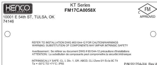
Figure 14: Intrinsically Safe Analog Output Label (Canada)
