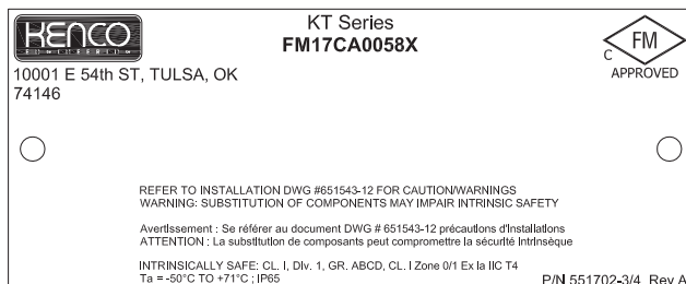
Figure 16: Intrinsically Safe Digital Output Label (Canada)
