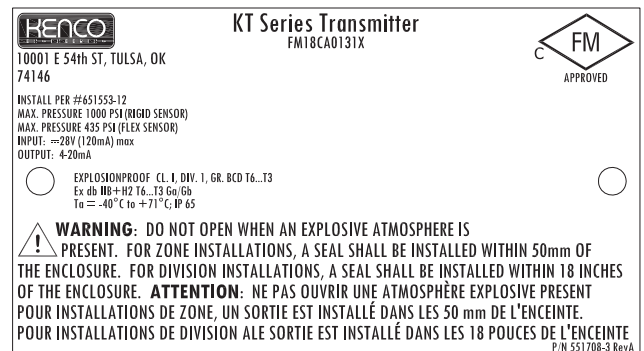
Figure 22: Explosion-Proof Analog Output Label (Canada) for 316 Stainless Steel Single Cavity Housing
